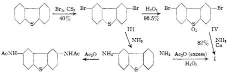
The 2,8-dibromo derivative (III) was obtained in 40% yield by long refluxing of a carbon bisulfide<sup>9</sup> solution of bromine and dibenzothiophene. The conversion to the dioxide (IV) was accomplished in almost quantitative yield by refluxing the sulfide with hydrogen peroxide in glacial acetic acid. Amination of the dibromo sulfone with concentrated aqueous ammonia and a trace of copper powder at  $175-220^{\circ}$  afforded the corresponding diamine.
